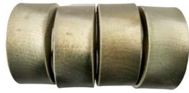
图6 焊接接头弯曲后试样 Fig.6 Specimens of the welded joint after bending
